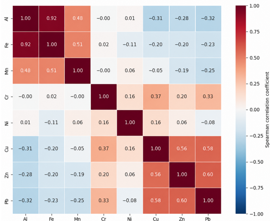
Figure 5. Clustered Spearman correlation matrix of selected elements in snowmelt samples collected in Pavlodar.
