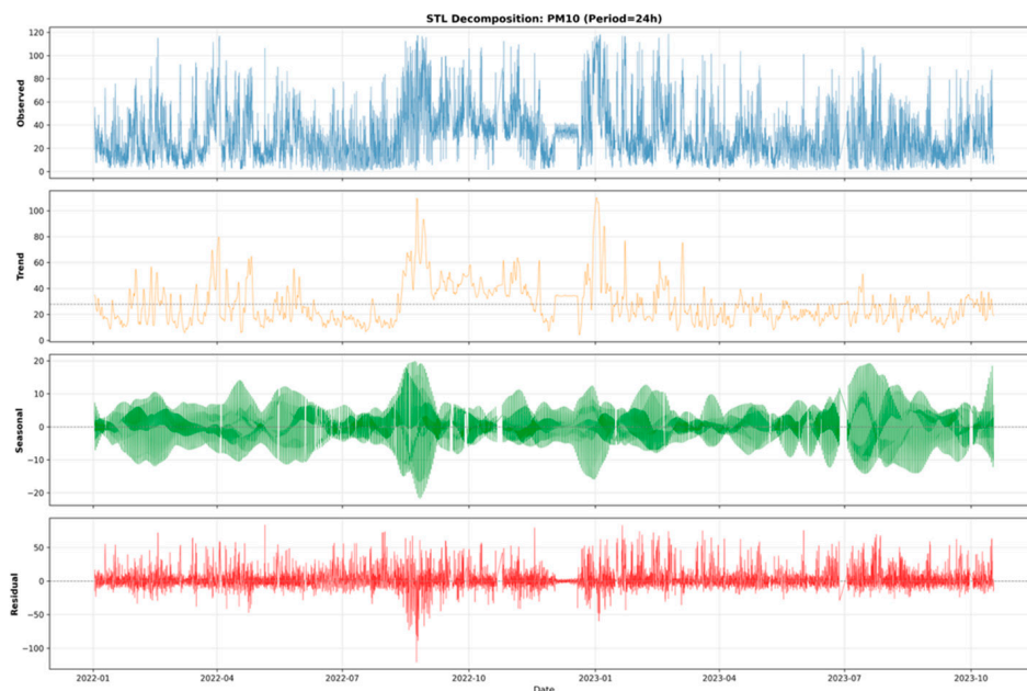
Figure 9. Decomposition of PM 10 Time Series into Trend, Seasonal and Residual Components by STL Method.
