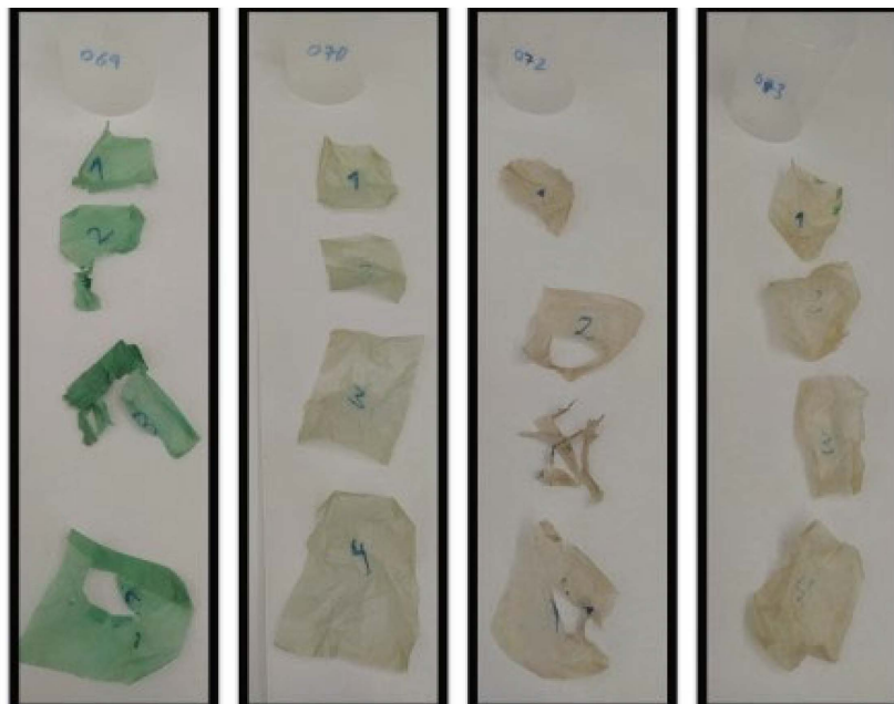
Figure 1. (A) Degradation of the 4 types of plastic films in vermicomposting systems, represented as % weight loss. Significant differences compared with the initial timepoint (T = 0) are indicated by *, while differences between vermicomposting systems are identified by #. (B) Visual appearance of sheets from each of the 4 types of plastics sampled after 120 days in a vermicomposting system with sewage sludge, post-washing and drying steps, from left to right: 069, 070, 072 and 073.
